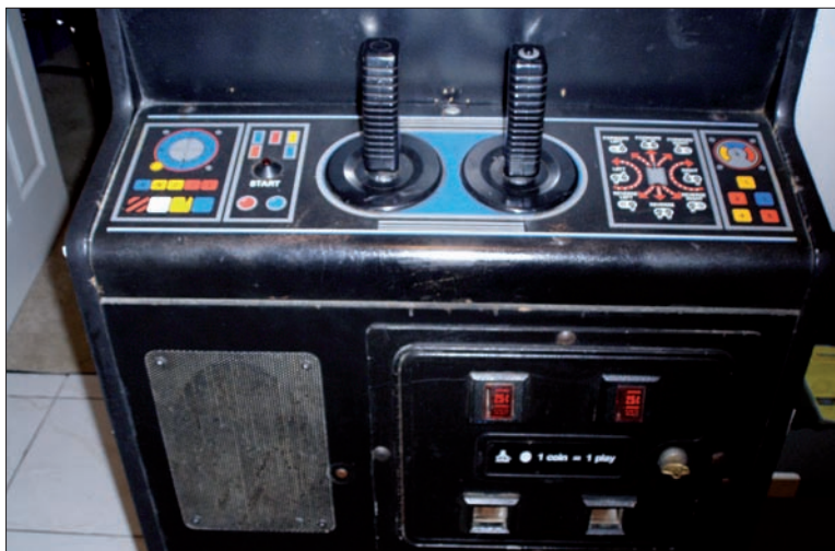
» Battlezone utilised a unique two-stick control system, with each stick controlling one of the tank's treads.
